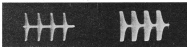
Fig. 2. Photographs of oscilloscope tracings of pulsed radiation; a. 25 % duty cycle; b. 50 % duty cycle
